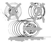
Your vehicle has anti-lock brakes, therefore apply the brakes steadily. Do not "pump" the brakes.
